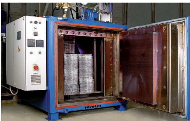
Anlassofen · Tempering furnace
